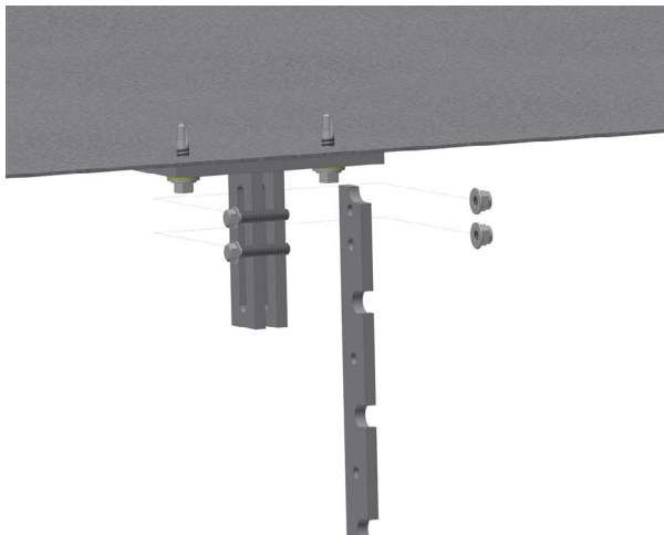
Fig. 24: Fixing pipe fixture
