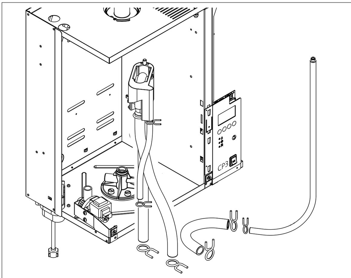
To improve accessibility for removing the water cup and the water hoses we recommend to remove the steam cylinder first (see chapter 7.3.1).
