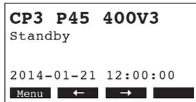
After the system test the unit is in **normal operation mode**. The display shows the **standard operating display** (first page of the indication level).
