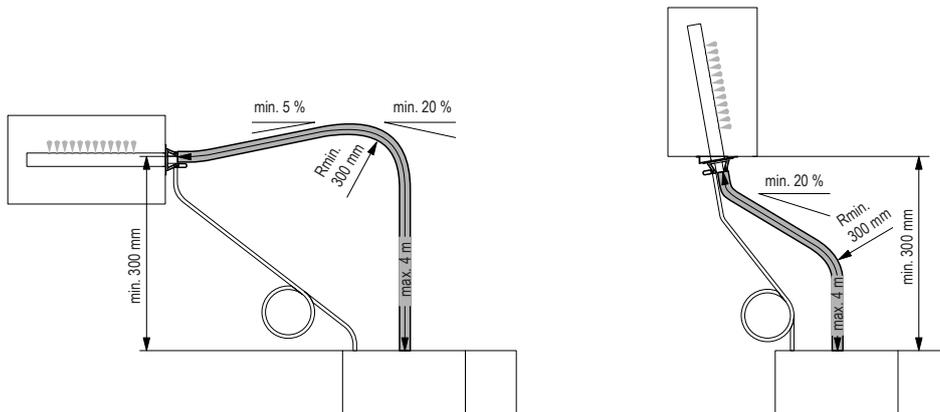
Initially, lead the steam hose with an **upslope of at least 20% over a minimum height of 300 mm**, then lead the hose with a **minimum upslope of 20%** and/or a **minimum downslope of 5%** to the steam distribution pipe.
