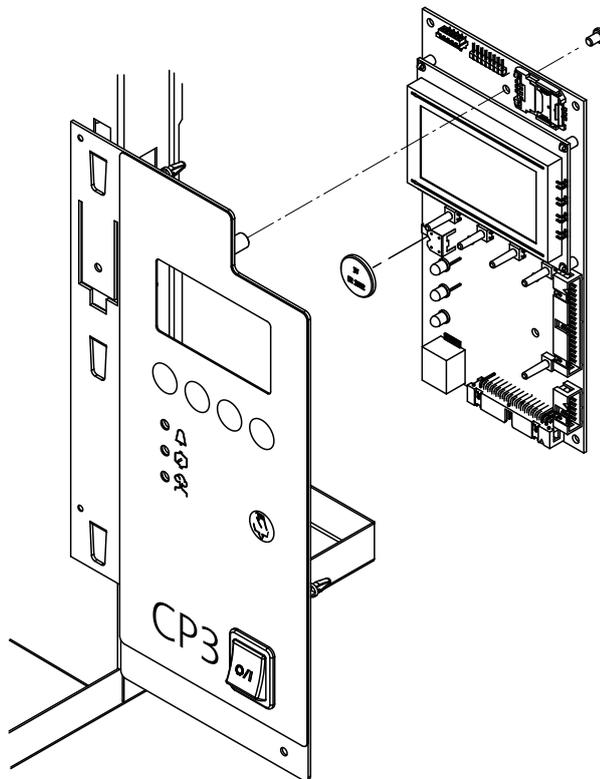
4. Undo the fastening screw of the control board, then carefully pull-off the control board from the control unit assembly.
