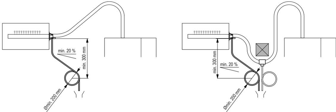
**Note:** If your unit feeds a number of steam distribution pipes, the individual condensate hoses are to be led into the discharge funnel.
