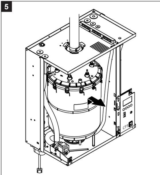
5. Carefully lift steam cylinder away from the cylinder receptacle, then remove it to the front.
