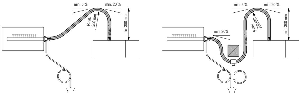
Initially, the steam hose is led with an **upslope of at least 20 % over a minimum height of 300 mm** above the top edge of the humidifier and then down to the steam distribution pipe with a **minimum slope of 5 %**.
