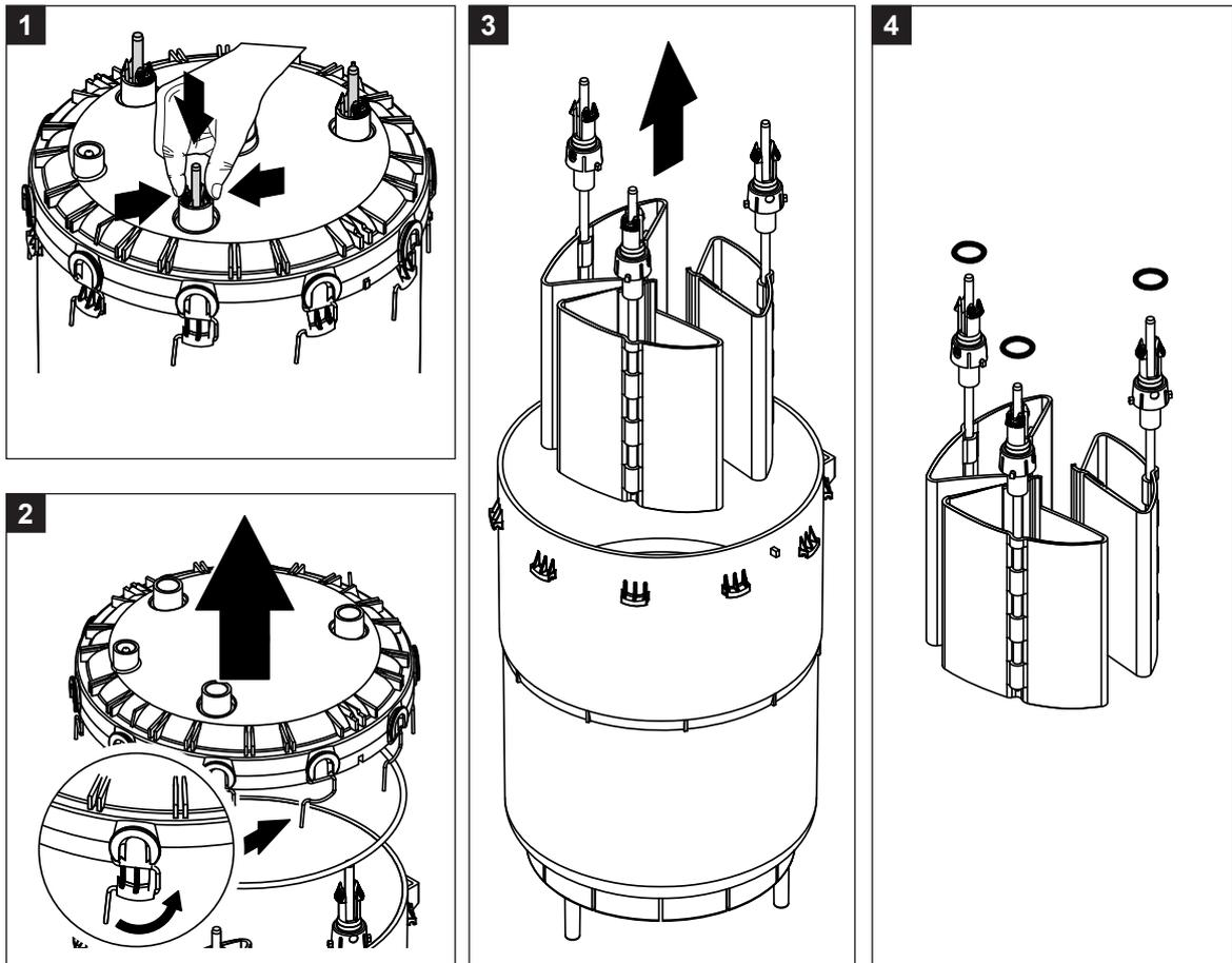
1. Fasten electrode snap fastenings and push electrodes approx. 2 cm downwards into the steam cylinder.
