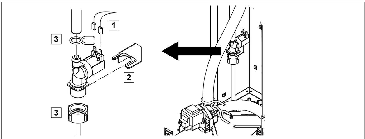
**The steam cylinder does not need to be removed** when removing the inlet valve.
