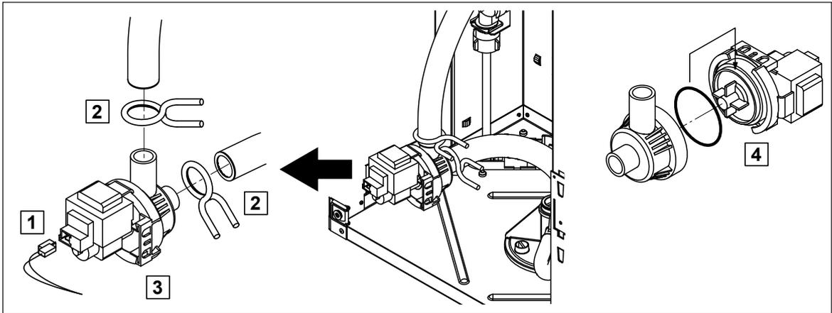
**The steam cylinder does not need to be removed** when removing the drain pump.
