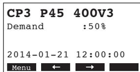
As soon as the humidity controller or the humidistat requires humidity, power is switched on for heating. The inlet valve opens (slight delay) and the steam cylinder fills with water. As soon as the submerged electrodes heat the water up the green LED lights up and after a few minutes (approx. 5–10 minutes, depending on the conductivity of the water) steam is produced.
